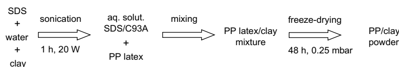
Scheme 1. The schematic representation of the multi-step preparation PP/clay nanocomposites by latex technology.
